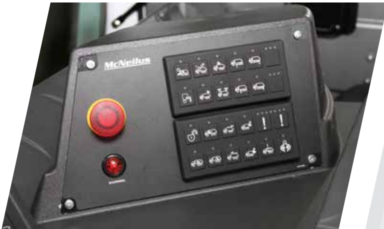
Command Zone Multiplex controls, integrated into the chassis cab
