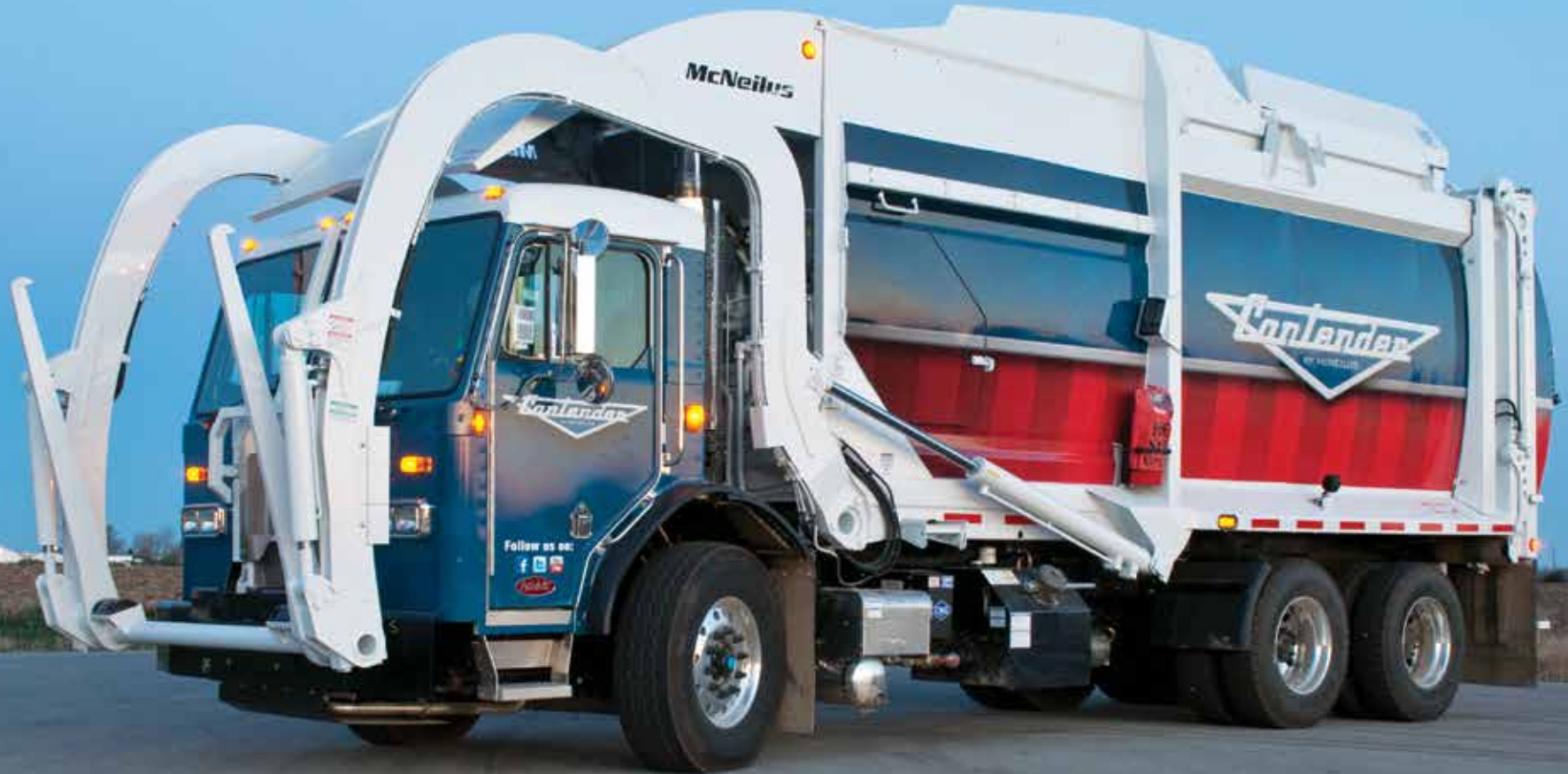
Contender with roof-mounted 60 DGE NGEN System
