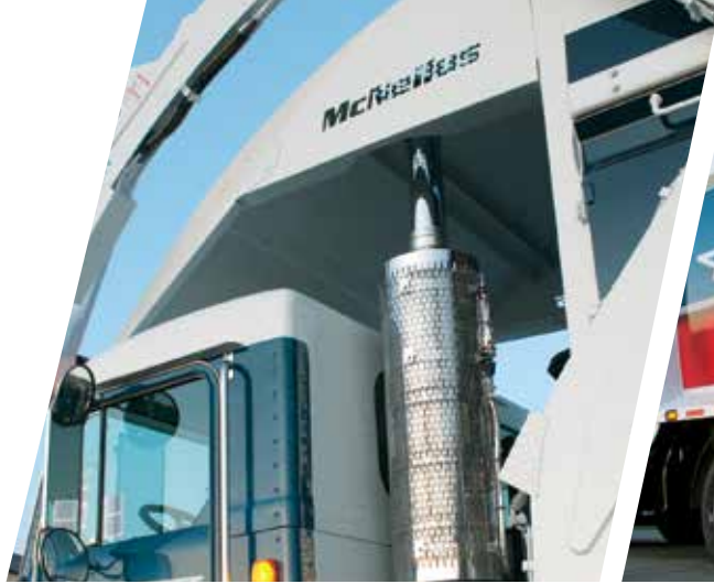
New hydraulic canopy offers excellent coverage on all chassis cabs.
